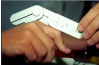
Figure 1. The EVAL electrogoniometer being used to measure the angle of the index MCP joint during grasp of a knife.
